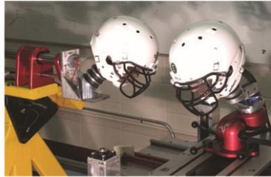
Videos used to guide laboratory reconstructions with mounted accelerometers
