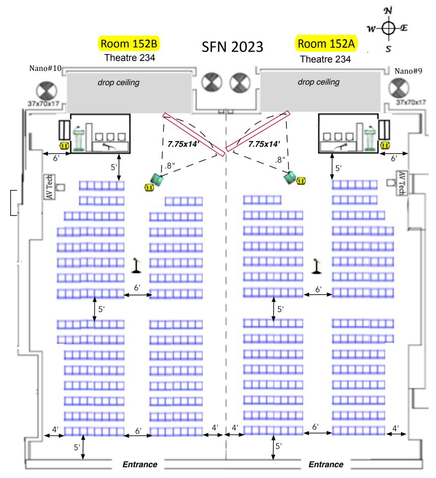
Audio: lect mic,tbl mics wireless HH (1), aisle mics (1) audio DI for computer playback
