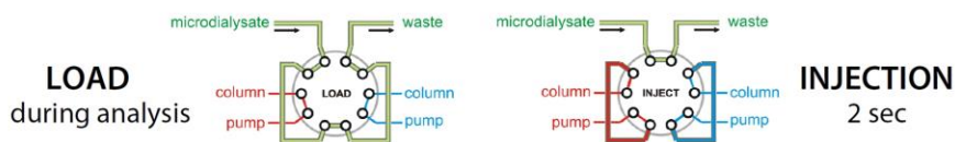
Figure 1. Schematic drawing of the set-up for online sampling & LC analysis.
