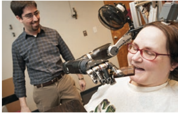
Figure 2. University of Pittsburgh clinical trial participant who has tetraplegia, resulting from spinocerebellar degeneration, neurally controlling a robotic arm to feed herself a bar of chocolate (Collinger et al., 2013). Photo courtesy of UPMC. Caution: Investigational device. Limited by federal law to investigational use.
