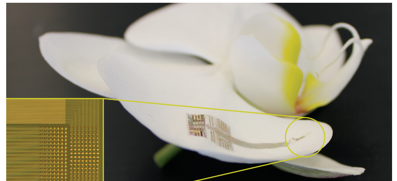
AN EARLY NEUROGRID, PLACED ON AN ORCHID PETAL TO ILLUSTRATE ITS CONFORMABILITY.
